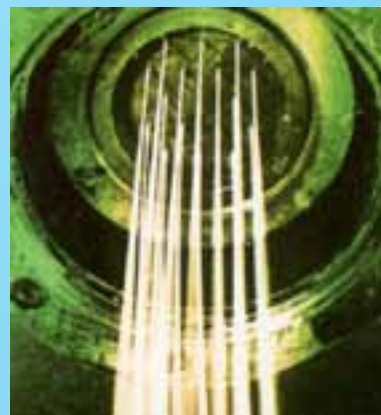
Synthetic fibers (like nylon and polyester) are extruded from a spinneret.
